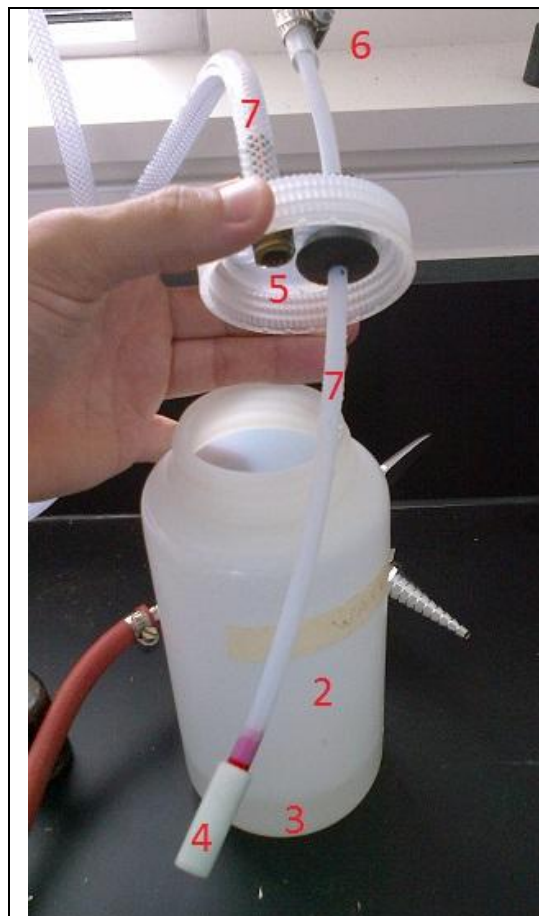
Figure 20: Airline Filtration System- Internal
